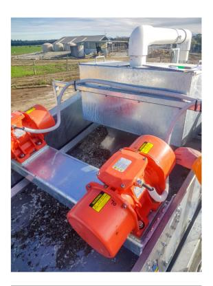
EMG calculated by changing to two smaller Oli vibrators the size and shape of the system could change alleviating the warping issue.
